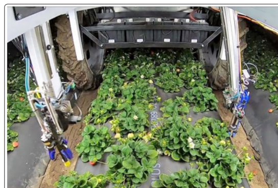
Figure 5: T-6 robotic harvester gently handles strawberries to avoid bruising and fruit damage.
