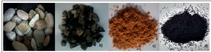
Figure 3: Materials used in the Filter: (a) Rolled Pebbles; (b) Gravel; (c) Sand; (d) Granular Activated Carbon (GAC).
