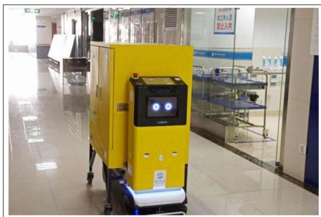
Figure 8: The Transfer Robot Carries the Empty Container to the Ward
