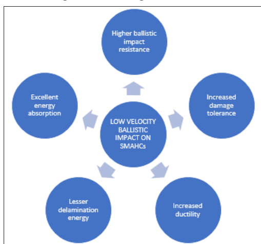
Figure 3: The advantages of shape memory alloy hybrid composites (SMAHCs) for the study of low velocity impact.
