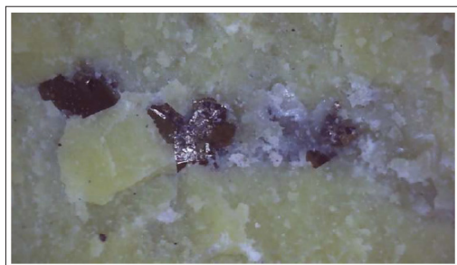
Figure 10: Veinlets of Chrysotile over the Figure 9 Sample Mineral, 25X (author’s Photograph)
