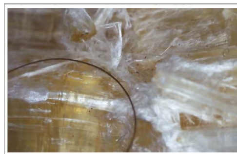
Figure 5: Chrysotile Fiber Group (Thousands of Tiny Fibers Packed Together) from Figure 4, 50X Compared to a Male Eyelash (author's Photograph)
