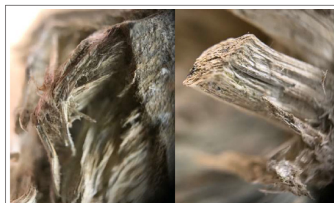
Figure 7: Chrysotile Fibers from Figure 6, 50X (author's Photograph)
