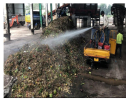
Figure 2: Dosing biological solution via spraying machine mounted on wheels
