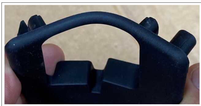
Figure 3: Part Molded with Sevrene 3000-70A Showing Excessive Flexibility
