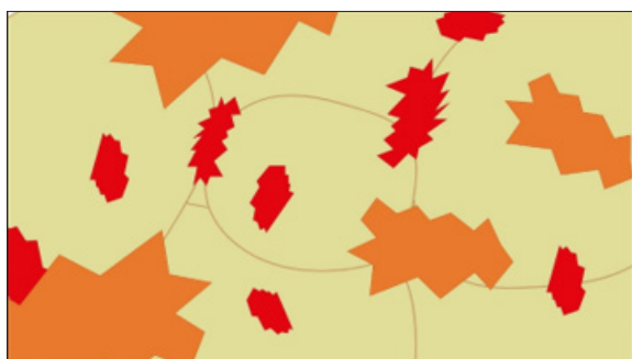
Figure 19: Model of Final Adhesion after Cooling from Sintering
