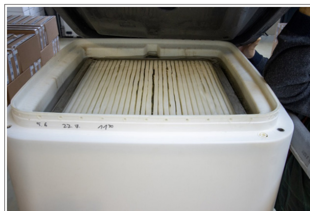
Figure 11: Prototype of a Water-to-PCM-Battery module at the top of a Buffer with 80 mm isolation [12]. The distance between the PCM-elements is 3 mm.
