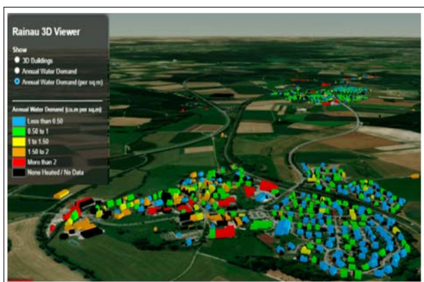
Figure 4: A 3D-Model of a Residential Area, Combined with Satellite Data, to Determine the Water Demand Per Building
