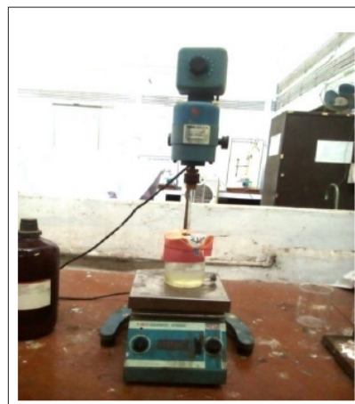
Figure 1: Experimental Setup for Kinetic Studies (Stirred Cell)
