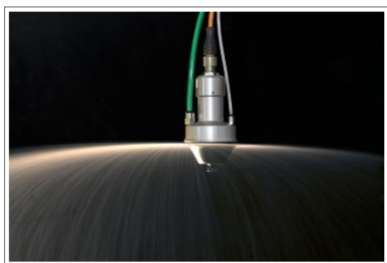
Figure 6: Rotary Atomiser for ULV Sprays
