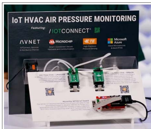
Figure 5: IoT Connect to Capture and move Pressure Sensor Data to the cloud and display it on a Dashboard
