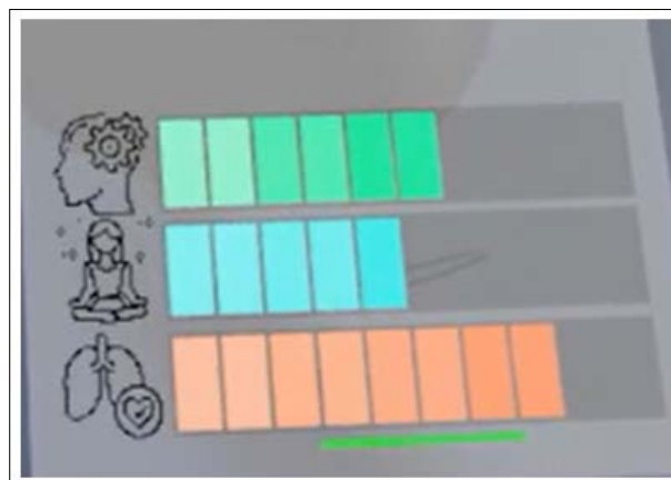
Figure 4: The small panel is displayed on the wrist of the virtual avatar, on which there are three icons representing three physiological measurements. The 3 biometric signals we have included here are: the eSense ® Attention metric, the first icon and the first bar from top to bottom, the eSense ® Meditation metric, icon and bars in the middle, and the physiological measurement of RSA or respiratory sinus arrhythmia which is referred to in the bottom bar.
